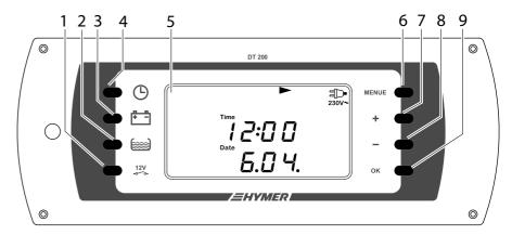
Fig. 1 Control and switch panel DT 200
