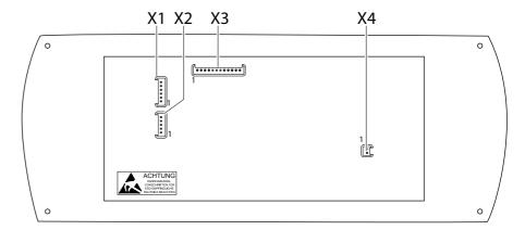
Fig. 6 Connection diagram for control and switch panel DT 200
